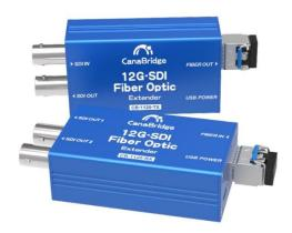
The CB-1120 12G-SDI Fiber Optic Extender is a transmitter/receiver kit supporting single-mode LC simplex fiber extensions up to 10km. It is a miniature-style extension solution that supports all SDI formats resolution up to 4K with audio and metadata. It features a local SDI loop out and dual SDI outputs and supports 12G/6G/3G/HD/SD-SDI signals.
